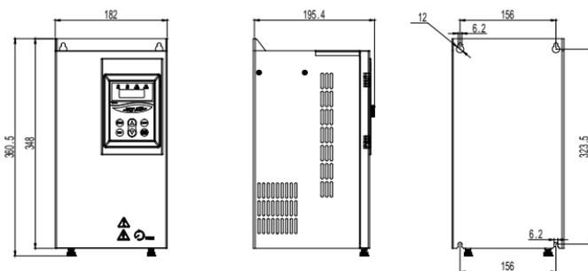
Figure 2-3 7.5-11kW Outline & installation dimensions diagram
