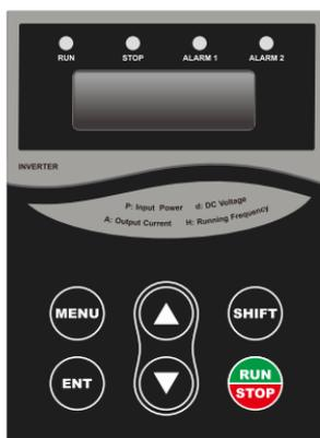
Figure 11 Keypad Schematic Diagram
