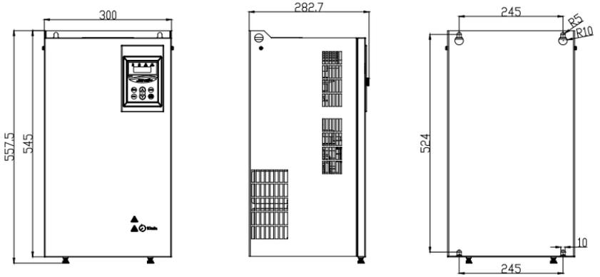
Figure 2-6 37-45kW Outline & installation dimensions diagram
