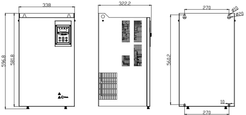
Figure 2-7 55-93kW Outline & installation dimensions diagram
