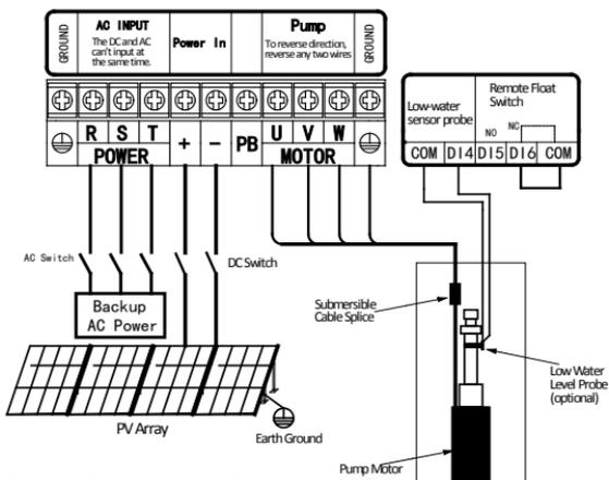
Figure 13 schematic diagram of alternate AC power supply
