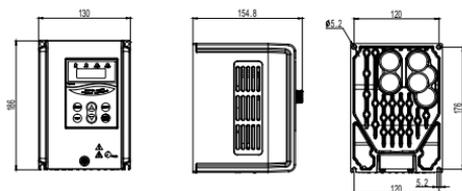
Figure 2-1 2.2kW Outline & installation dimensions diagram
