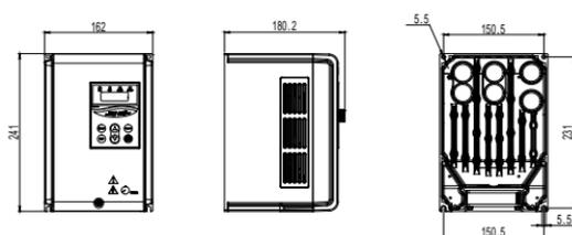
Figure 2-2 4-5.5kW Outline & installation dimensions diagram
