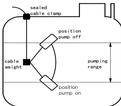
Figure 8 Floating Ball Diagram
