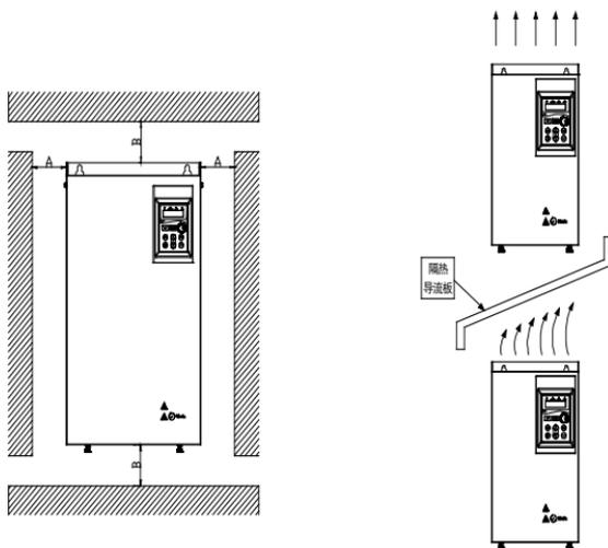
Figure 4 Ventilation Arrangement and Required Distances
