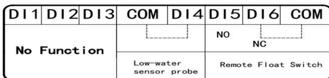
Figure6 Control terminals (The sequence may be different from actual product)
