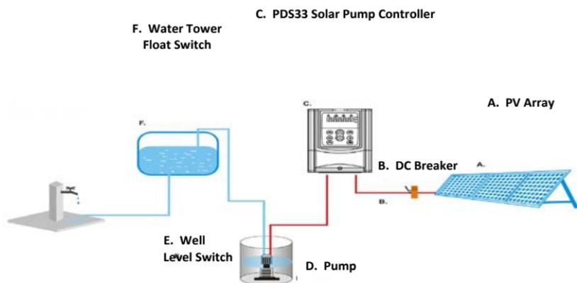
Figure 1 PDS33 solar pumping system
