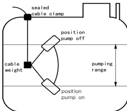
Figure 8 Floating Ball Diagram
