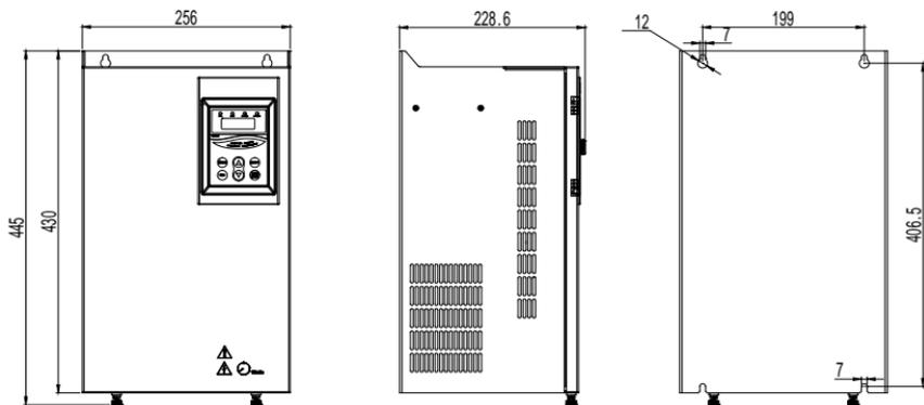
Figure 2-5 22-30kW Outline & installation dimensions diagram
