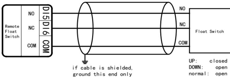
Figure 9 Float ball wiring diagram
