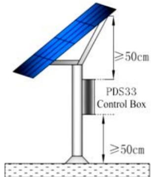
Figure 3 Control Box Location
