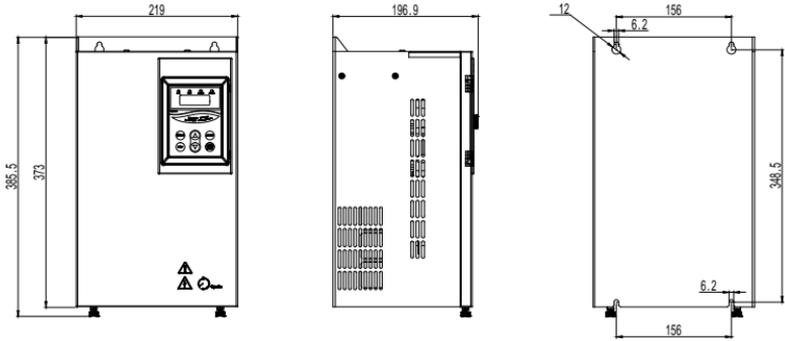
Figure 2-4 15-18.5kW Outline & installation dimensions diagram
