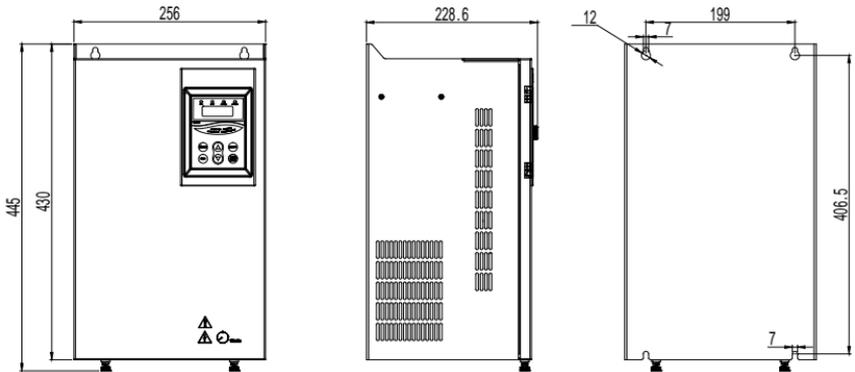
Figure 2-5 22-30kW Outline & installation dimensions diagram
